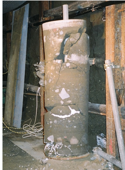
Photo 2. Specimen retrieved after test (C-1)
