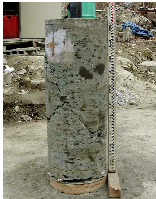
Photo 1. Specimen retrieved after Test 2 (Tani, 2003)
